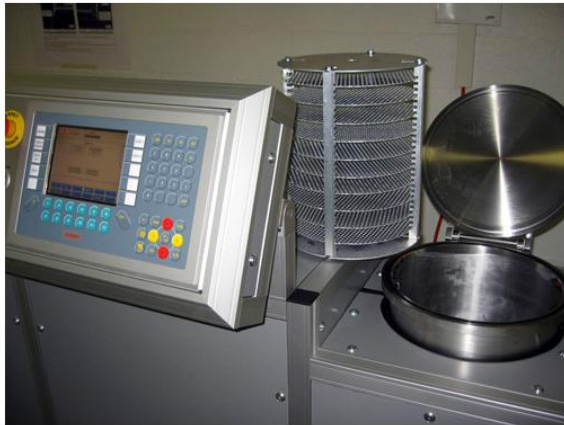
Parylene front panel, 10 slots holder and processing chamber
