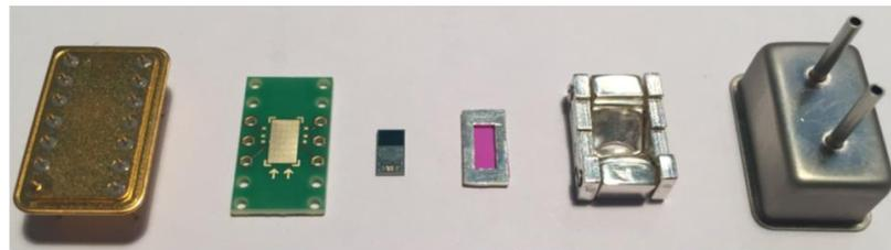
socket      PCB      MORES Chip      sensitive layer and frame      reflector module      housing with gas in- and outlet
