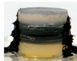
Energy harvester Stack of 128 layers 5 mW in 1 cm 3
