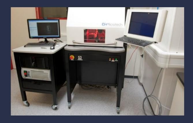
Laser soldering & welding station in cleanroom environment
