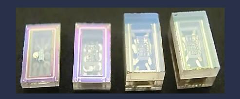
4 different designs with rad hard materials Sapphire with and w/o lens Schott N-BAF4 & N-ZK7 type glasses
