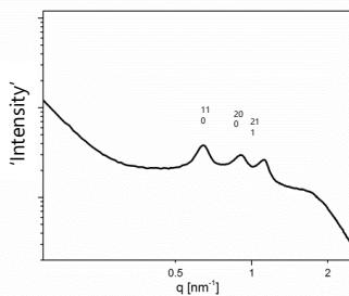
Angular intensity patterns help identify internal structures. The three characteristic peaks belong to Im<sub>3</sub>m Cubic Phase!
